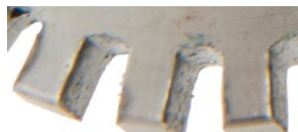
Competitive hub shows pitting on teeth and burrs on tooth edges from broken grid element.
