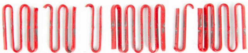
Dodge** grid element after 70,000 cycles
